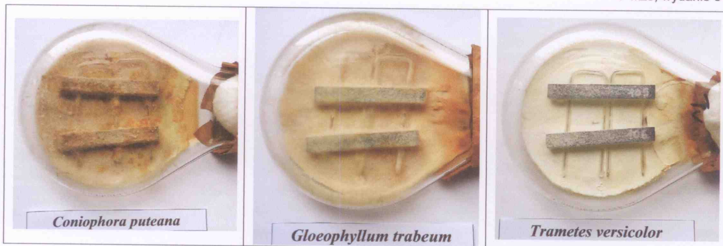
Photo 2. The overgrowth of samples by fungi at the end of the test.
